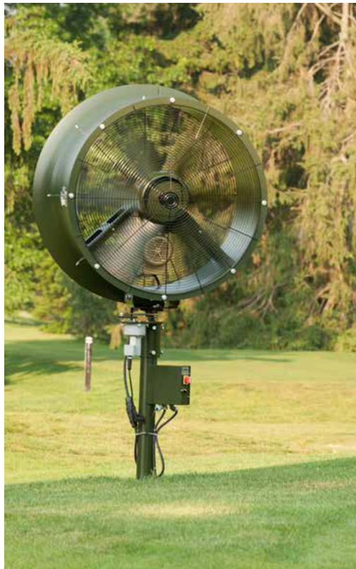
Figure 21. Fan used to cool low cut turfgrass surfaces. Photo courtesy of GCSAA.
