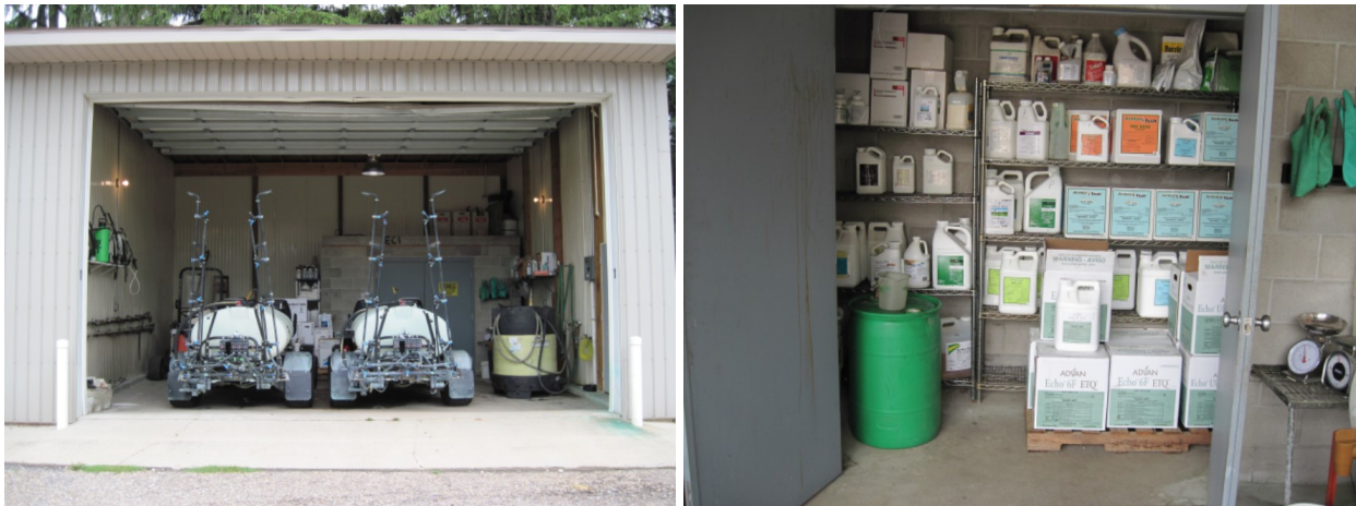
Figure 5. Separate building for storing, mixing and loading plant protectants complete with metal shelving for chemicals in a locked, limited access area, at Elcona Country Club. Photos courtesy of Ryan Cummings.
