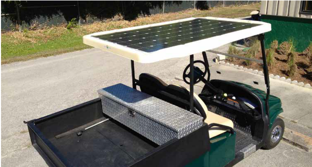
Figure 23. Use of solar panels to power a utility cart. Photo courtesy of GCSAA.
