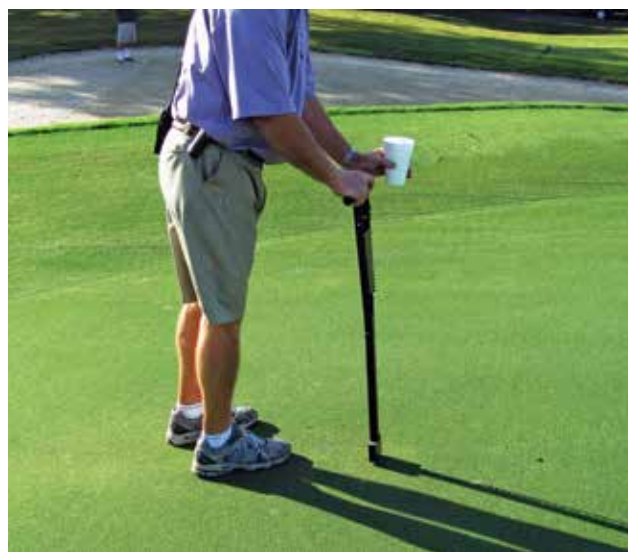
Figure 3-3. Using a highly accurate TDR probe to measure soil moisture levels.
