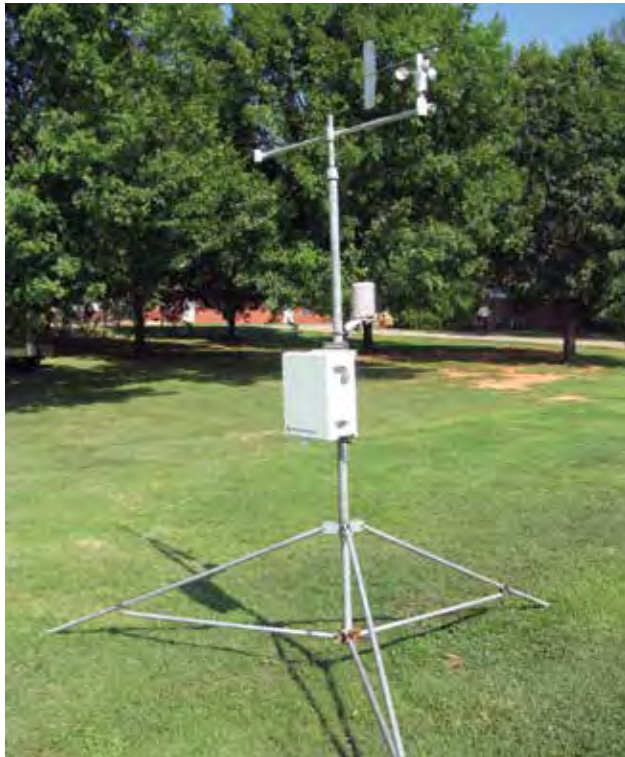
Figure 3-4. An on-site weather station which measures environmental conditions which in-turn are used to predict irrigation needs.
