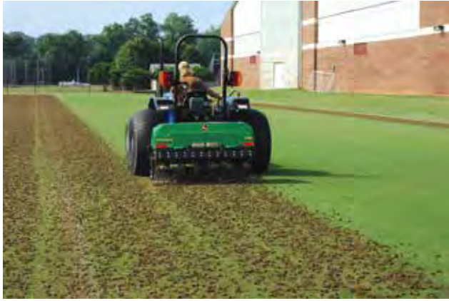
Figure 5-8. The only practical means with which golf courses can relieve soil compaction is aerification followed by cores being discarded.
