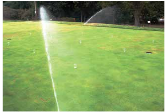
Figure 3-5. Using a 'jar-test' to accurately measure the distribution uniformity of an irrigation system.
