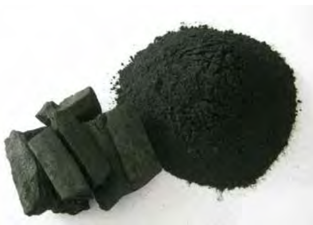
Figure 11-10. Activated charcoal has a wide array of uses such as deactivating unwanted pesticide applications or for artificially warming soils.
