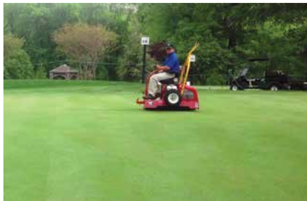
Figure 5-21. Use of a roller to help smooth the playing surface and to increase ball roll distance.
