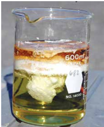
Figure 11-5. When unfamiliar with mixing products, a jar test should be performed to ensure they are compatible.
